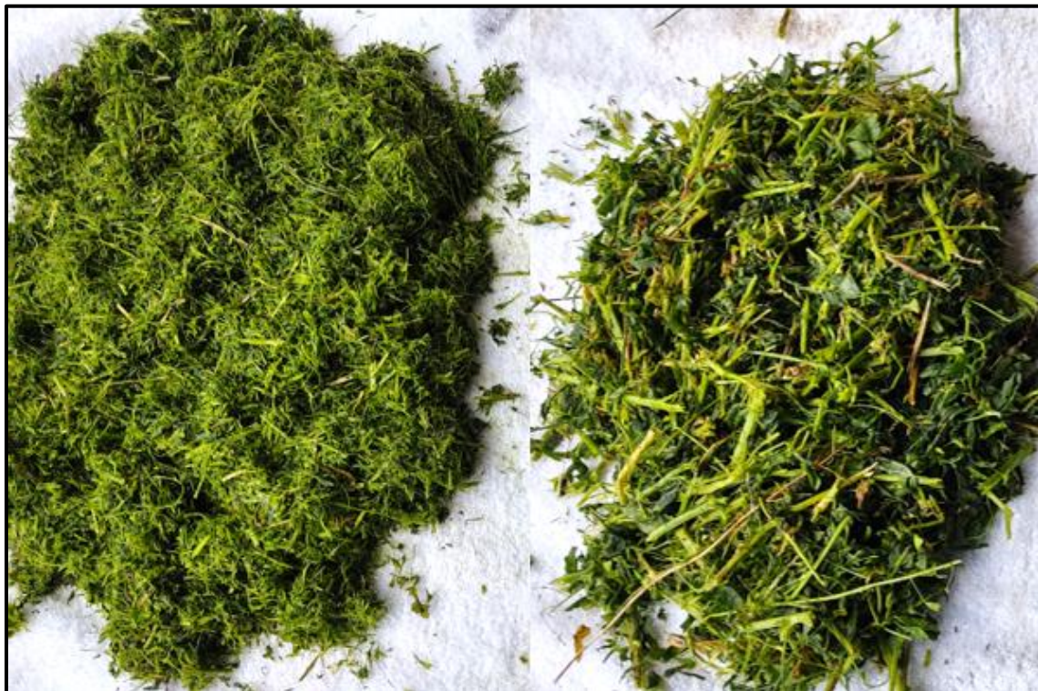
Figure 2. Example of chopped material (right) and processed material (left). Note that processing shreds and fiberizes the stems.
